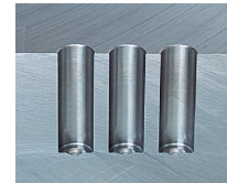
ワーク材質：金型調質鋼 (40HRC) 断面 Work piece: Quenched and tempered steel (40HRC)
